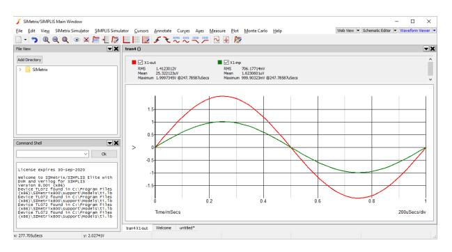
To remove the measurements, use menu *Measure > Delete All Measurements*. Alternately to remove specific measurements, make sure only a single curve is selected then use menu *Measure > Delete Measurements...* and choose the measurements to remove.
