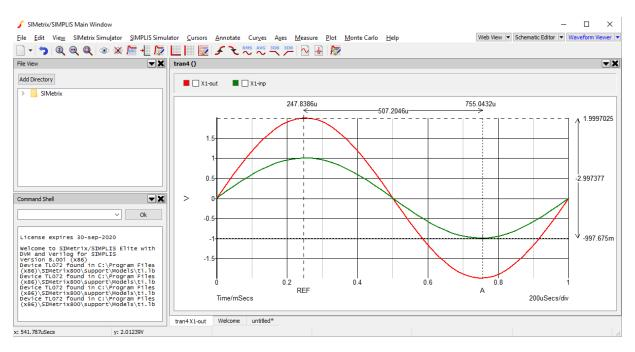
Next we'll also measure the minimum of X1-out and compare this to the maximum of X1-out. Instead of moving our cursor A, we will add a new cursor, so then we can see the two difference measurements at the same time.
