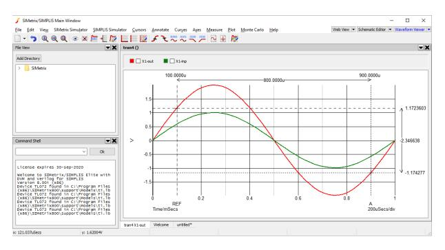
Initially we are provided with two cursors, labelled *REF* and *A*, these labels can be found on the x-axis. The cursors are positioned at two points on a curve, the points are by default placed at the intersection of the vertical line going up from the label name and the horizontal line with the same line-style. The cursors are visually shown with a horizontal-vertical cross at this intersection.
