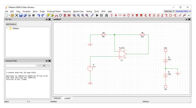
Now we need to add matching connectors to the supply rail of the op-amp. First select the +5V connector by clicking on it, then press the duplicate button (or the default shortcut Control-D). The cursor will show the outline of a connector, move and rotate it as required to place it next to the +ve supply rail of the op-amp. Repeat this for the -ve supply and wire the new connectors to the supply rail pins on the op-amp.
