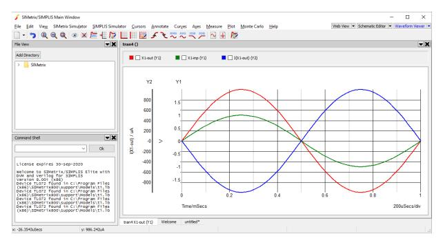
We can now see that a second y-axis has been added. Additionally, the y-axis being used by each curve is now also displayed in the legend box in brackets.
