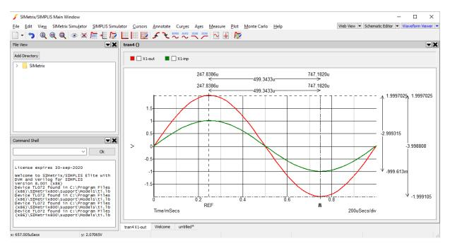
When multiple cursors are placed on the waveform, multiple measurement indicators are shown alongside the waveform. In this case it allows us to read-off the voltage differences between the two curves as 3V and 4V respectively.
