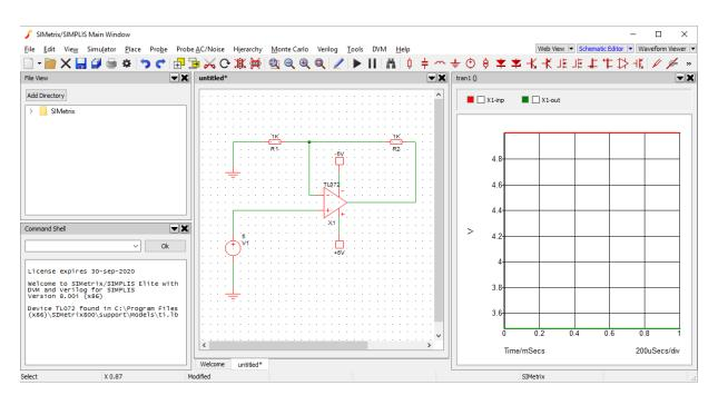
This is clearly a fairly boring simulation that has been run, as the input voltage has remained constant throughout. So we will need to adjust the parameters on the voltage source.
